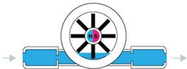
Fig. 7. YF-S201 Hall transducer operation
